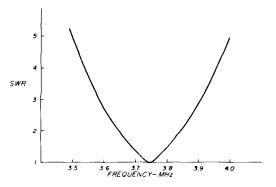
fig. 3. Calculated SWR of the dipole equivalent circuit.
